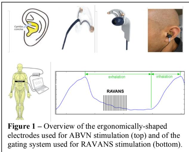
**Figure 1** – Overview of the ergonomically-shaped electrodes used for ABVN stimulation (top) and of the gating system used for RAVANS stimulation (bottom).
