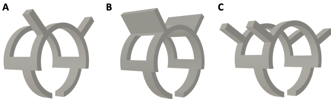
Figure 17: Easy-open Helmet. 320° arch with two bars in the upper half including each of them two vertical bars to ease the opening of the piece.
