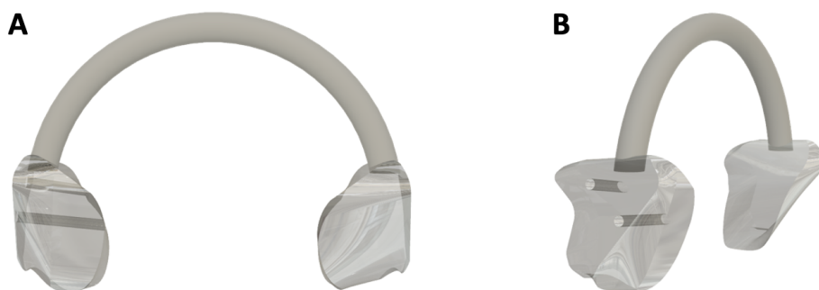
Figure 14: Concept of headphones. Structure including two pods built as depicted in 2.2, and a plastic arch as a uniting piece; (A) frontal view (B) diagonal view
